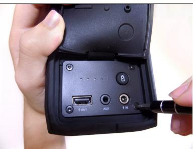
Turning the device on its side, unscrew the four 15mm hexagon 2.0 screws on the charging port panel.
