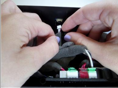
• Unplug the wire on the inside of the device that connect to the button panel.
