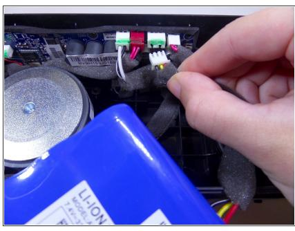
from their ports. The metal stems attached to the ports can break. A spudger or tweezers may help.
