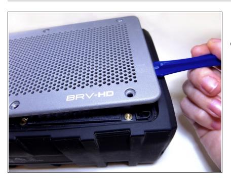
Lift the front panel off of the speaker using a plastic opening tool.
