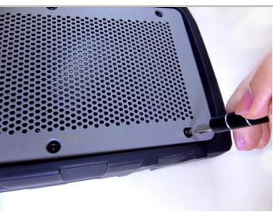
Placing the device with the back panel facing up, remove the eight 5mm hexagon 2.0 screws from the back panel.
