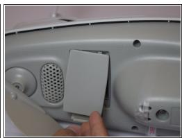
Remove the battery compartment lid by lifting upward.
