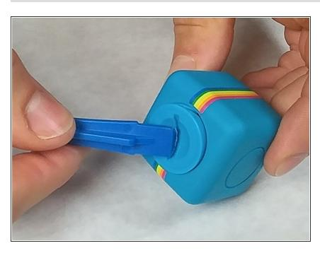
Remove the SD card cover by twisting it using a Plastic Opening Tool
