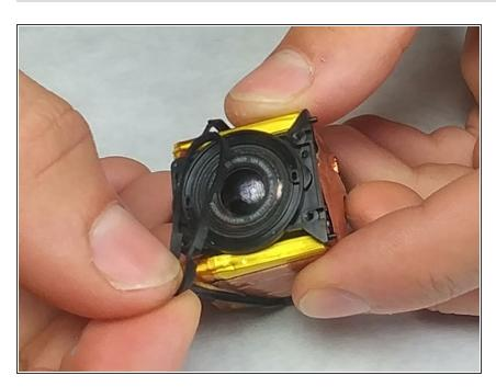
Remove the rubber seal wrapped around the camera.
