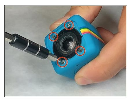
Using a J00 head screwdriver, remove the four 3.27mm screws from the front of the camera near the lens.
