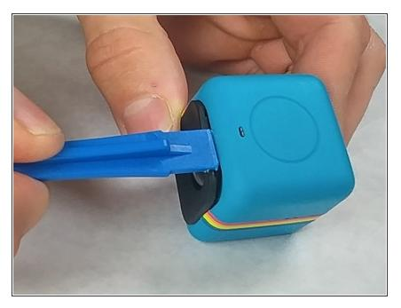
Use the Plastic Opening tool to pry off and remove the front cover.
