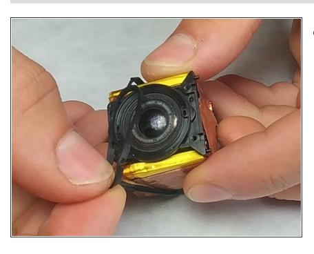
Remove the rubber seal wrapped around the camera.
