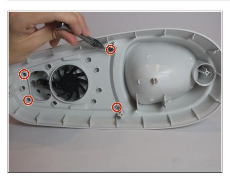
Remove the four 0.8cm screws inside the case located near the fan using the J1 screw bit.
