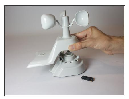
Carefully slide apart the two parts of the solar panel housing.
