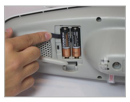
Pull the ribbon to eject the 2 X AA alkaline batteries.
