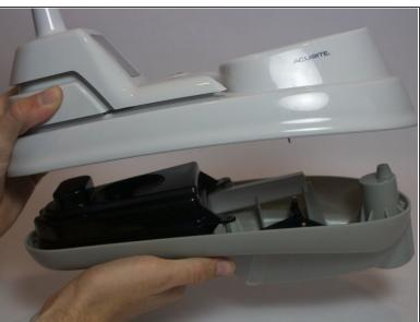
Gently lift the top section of the weather center away from the base. With all the screws removed it should lift off easily.
