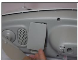
Remove the battery compartment lid by lifting upward.
