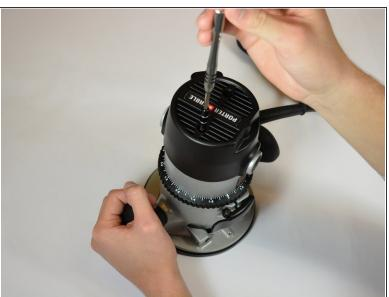
Use a Torx screwdriver to unscrew the 25.4 mm screws found at the top of the model.
