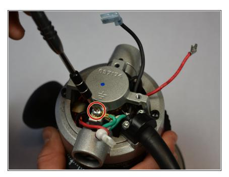
Use a pentalobe screwdriver to unscrew the 11 mm screw.
