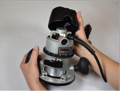
Remove the top by gently lifting the cover from router body.
