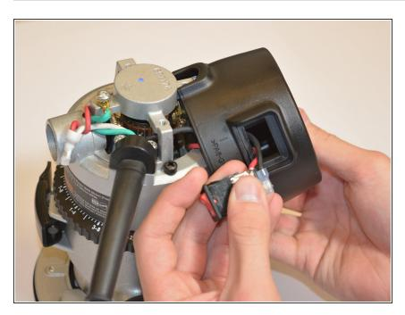
Push the power switch through the top of the router. The power switch should now be completely detached from the router (besides the wire connections).
