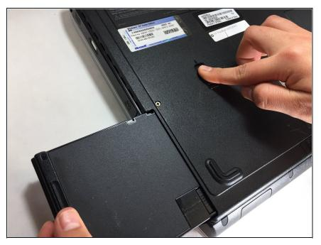
While continuing to push upward on the switch, slide the battery out on the left side of the laptop.
