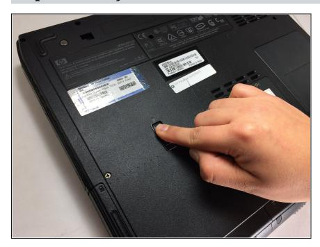
Push the battery release switch upward.
