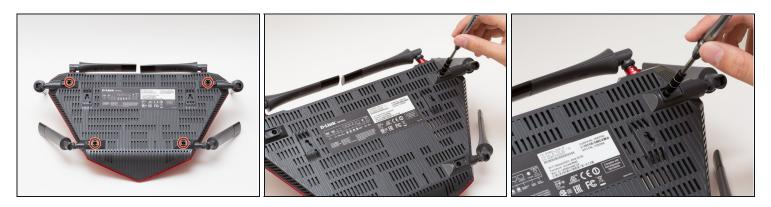
Unscrew the 5mm screws in each corner using the Phillips #1 screwdriver.
