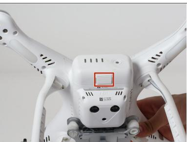
With the battery facing you, locate the two tabs on the top and bottom of the battery as shown.
