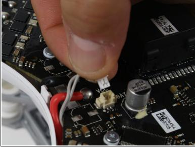
Remove the cable next to where the battery wires were connected. Pinch and hold the top of the connector, then pull it out.
