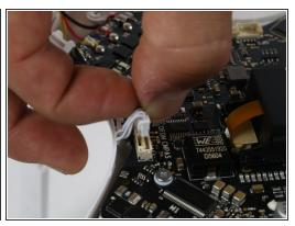
Remove the black ribbon cable and the 3-wire cable next to it. Press the small tab on the ribbon cable connector and pull it out.
