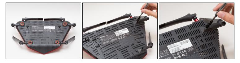
Unscrew the 5mm screws in each corner using the Phillips #1 screwdriver.
