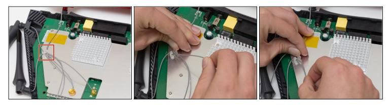
• Open the plastic bracket enclosing the three antenna wires and pull the wires out with your hands.
