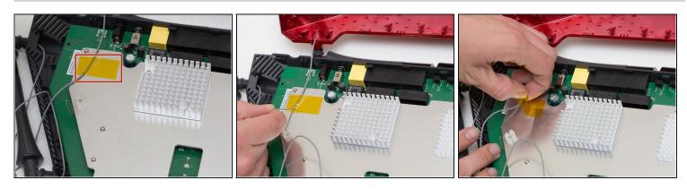
• Pull the yellow tape off of the motherboard to release the final antenna wire.
