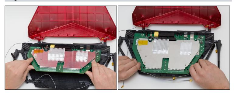
• Pull the the motherboard away from the case to remove it. Start on the side closest to you, and pull up and out.
