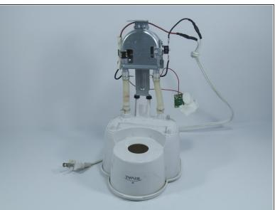
Flip the device upside down and remove the outer plastic body from the device by pulling straight up.
