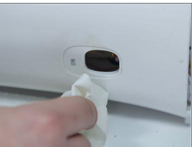
Clean both the button and its slot before replacing the power button.
