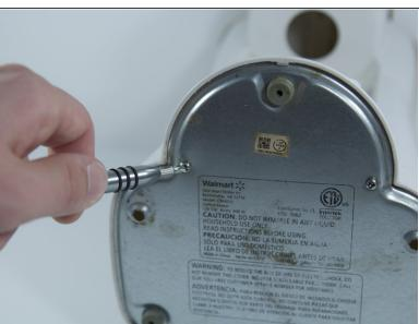
Remove the three 16 mm tri-point screws from the base plate.
