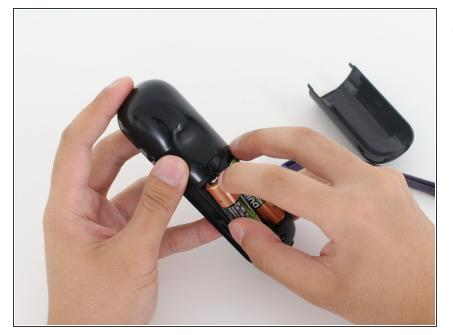
Remove the batteries by placing a finger on one end of the battery and pushing downward while pulling the battery out.
