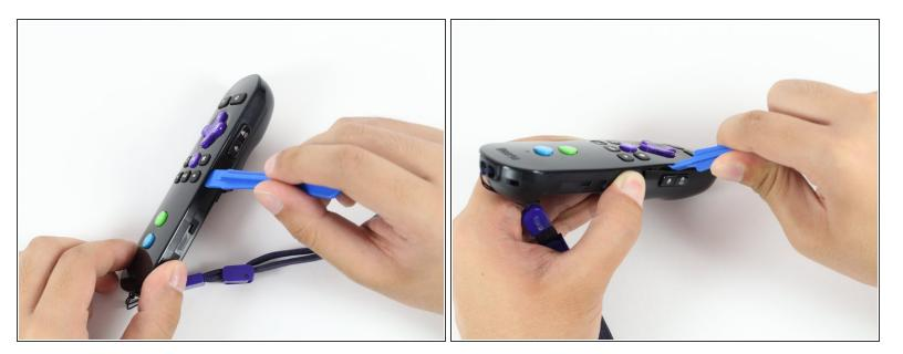
• Gently pry open the remote using the plastic opening tool.
