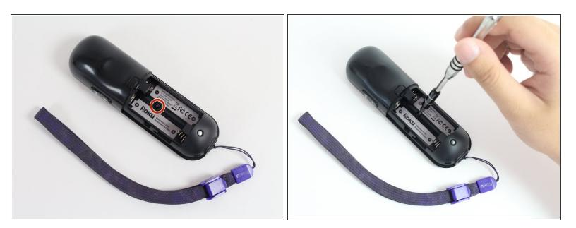
Unscrew one 7 mm Phillips #0 screw from the center of the battery compartment.
