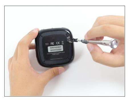
Remove the 9 mm screws from the three corners with a Hex 1.3 Screwdriver.
