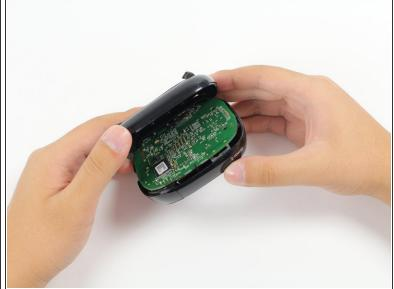
Open the device by gently lifting the bottom half away from the top half of the device.
