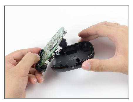
Use your fingers to carefully lift the motherboard from the top half of the device.
