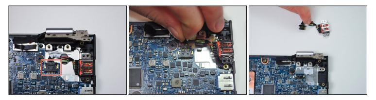
• Carefully slide bundle cable connector out from its connector on the motherboard.
