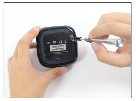
Remove the 9 mm screws from the three corners with a Hex 1.3 Screwdriver.
