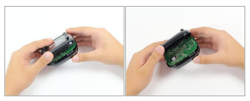
• Open the device by gently lifting the bottom half away from the top half of the device.
