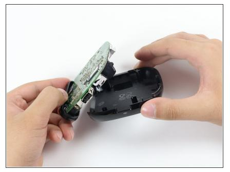
• Use your fingers to carefully lift the motherboard from the top half of the device.
