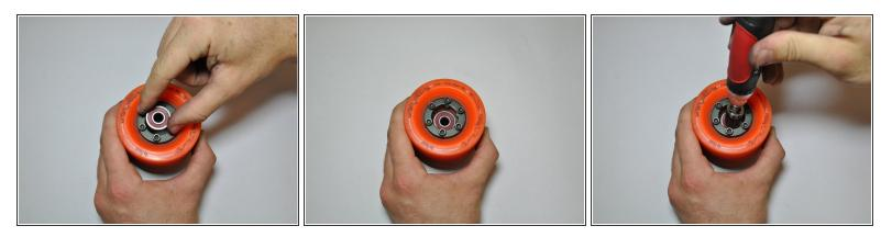
Replace bearing by dropping it in the center of the wheel and use a socket wrench to pop in back it place
