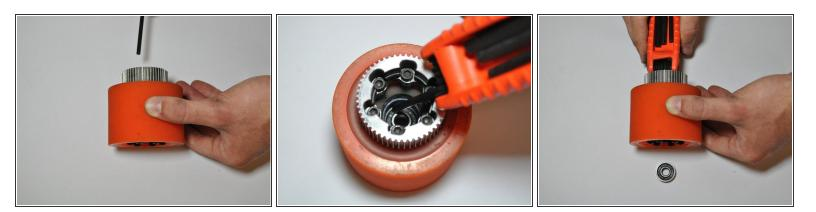
• Use an Allen wrench to apply pressure to the inside edge of the bearing until it pops out
