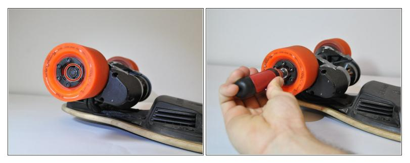
Remove the axel nut with a 1/2" socket wrench
