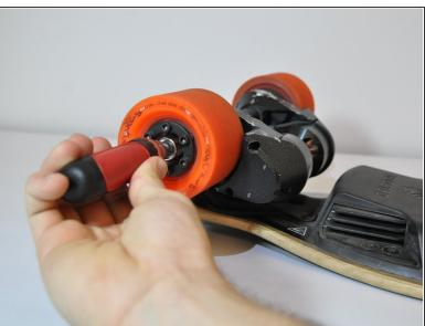
Remove the axel nut with a 1/2" socket wrench
