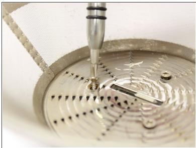
To remove the cutting disc, unscrew the three Phillips #1 screws.
