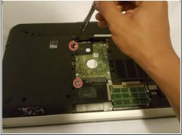
Locate and remove the four 4mm screws holding the hard drive in place.
