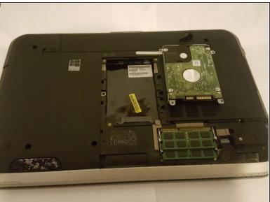
Lift the hard drive up and out of the bay.
