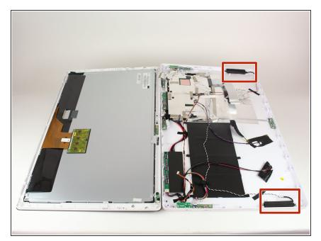
Locate the faulty speaker. The two speakers are located in the upper corners of the back panel.
