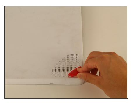
Use your fingers to carefully peel them off the device to reveal the screws underneath.
