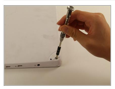
Use a Phillips #1 screwdriver to remove the 9.5 mm screw in each of the four corners.
