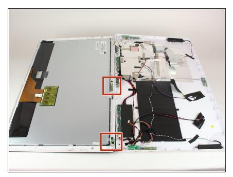
Locate the two cables running on both sides of the device found at the bottom side of the screen.
