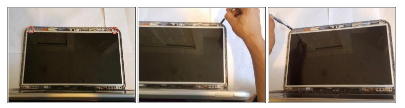
• Locate and remove the top two 4mm screws.
