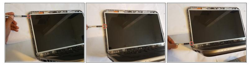
• Locate and remove the three 3mm left hand side screws.
