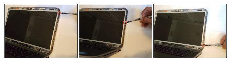
• Locate and remove the three 3mm right hand side screws.
