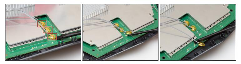
Pry off the antenna connectors using a heavy-duty spudger.
