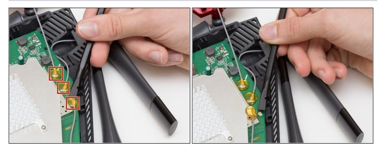
• Continue to pry off the last three antenna connections on the upper right portion of the motherboard.
