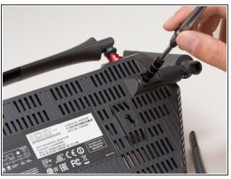
Unscrew the 5mm screws in each corner using the Phillips #1 screwdriver.
