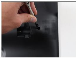
Remove the 4 screws (4 mm in length) using the Phillips #0 screwdriver.
