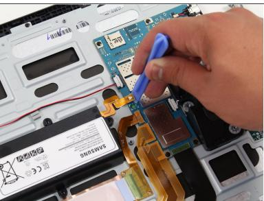
Using the plastic opening tool, lift off the orange press-fit connector (marked with a white arrow-head) where it attaches to the motherboard.
