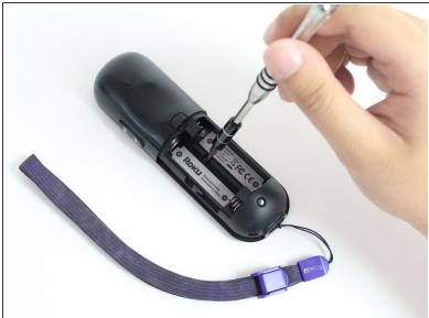
Unscrew one 7 mm Phillips #0 screw from the center of the battery compartment.
