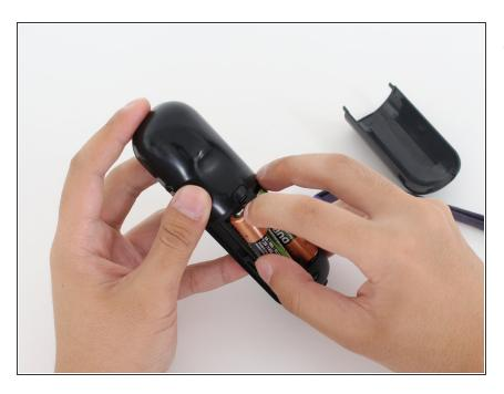
Remove the batteries by placing a finger on one end of the battery and pushing downward while pulling the battery out.
