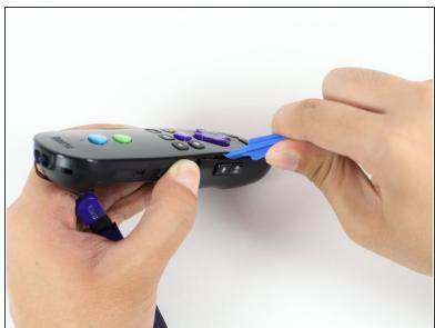
Gently pry open the remote using the plastic opening tool.
