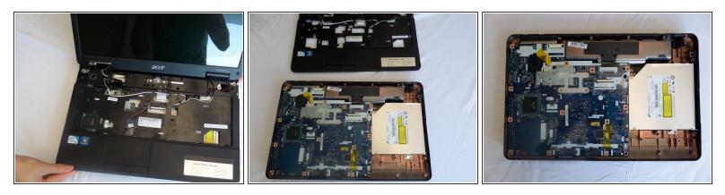
• Flip to the front and gently lift the front of the laptop off of the base.
