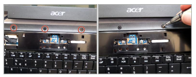
• Remove the three screws with a #00 Philips Screwdriver.
