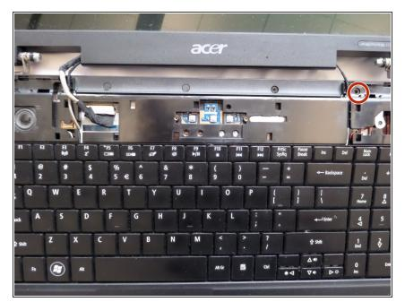
Remove the single screw next to the right hinge with a #00 Phillips Screwdriver.
