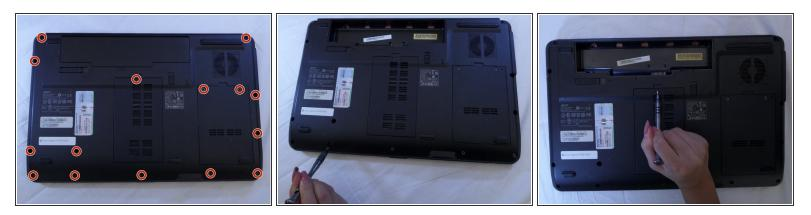
• Remove the fifteen screws from the back of the laptop with a Phillips #00 Screwdriver.
