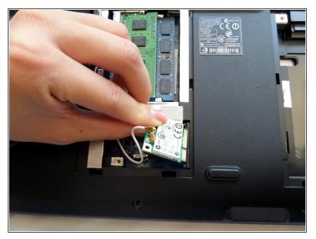
• The small circuit board will pop up easily. Carefully remove it
