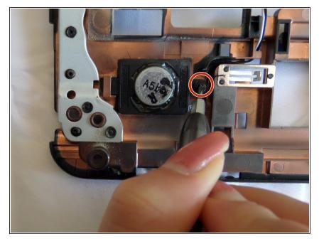
• Using a Phillips #00 screwdriver, remove one 2.5 mm screw to loosen the speaker from the panel.
