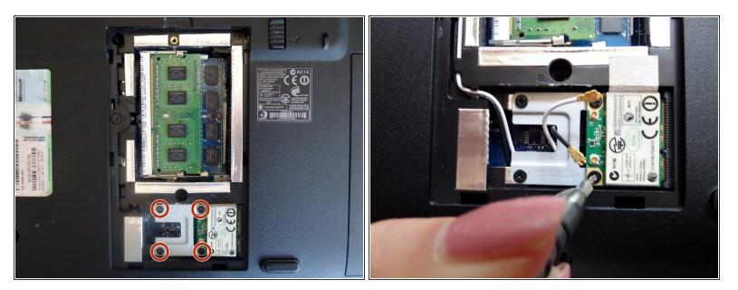
• Remove the four screws from the metal piece beneath the circuit with a Phillips #000 Screwdriver.
