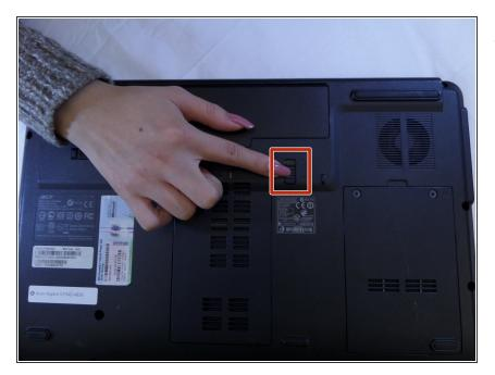
Slide the right latch down to unlock the battery.
