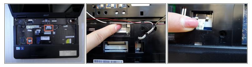
Disconnect the two blue and white ribbons by applying pressure downward and pushing them out of their sockets.
