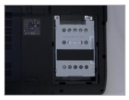
• Lift the hard-drive cover in the bottom right corner off the laptop.
