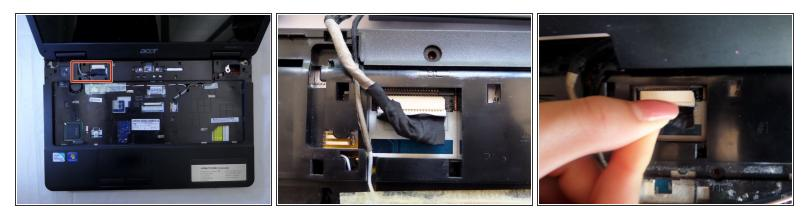
Disconnect the screen connector in the upper left of the laptop.
