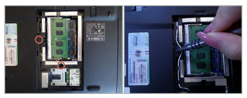
• Remove the two screws on the left and bottom of the circuit board with a #00 Phillips Screwdriver.
