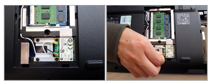
Disconnect the black and white wires on the small circuit board by gently pulling them out of their sockets.
