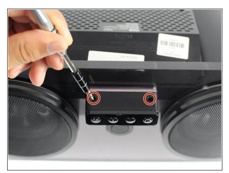
• Remove the two 9.5 mm Phillips #1 screws from the dock cover.
