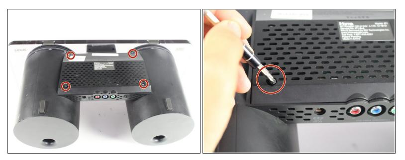
Remove the four 9.5 mm Phillips #2 screws located on each of the four corners of the iHome's back cover.
