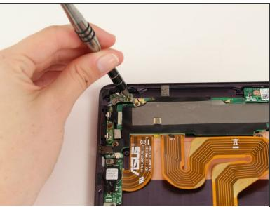
Remove the two 2.5mm screws using a Phillips #00 screwdriver.
