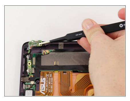
The electronic portion of the lock and volume buttons should now be free to move. Lift it gently using tweezers, and set it aside.
