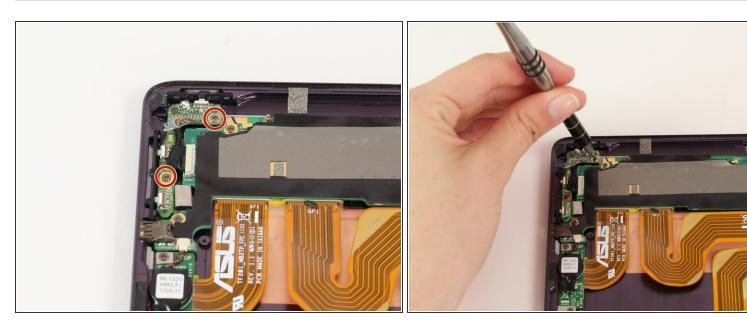
Remove the two 2.5mm screws using a Phillips #00 screwdriver.
