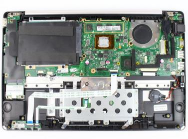
Grab the sides of the fan assembly and remove it by lifting upwards.
