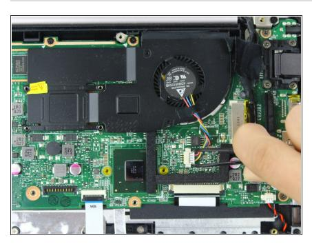
Disconnect the fan's power cable by pulling upward on the pin connector with a pair of tweezers.
