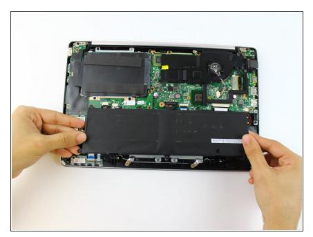
Lift and remove the battery.
