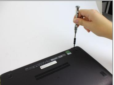
• Use a Phillips 0 screwdriver to remove nine Phillips screws from the back of the laptop (four 7mm from the top hinge, four 5mm from the bottom hinge, and one 10mm screw from the center).
