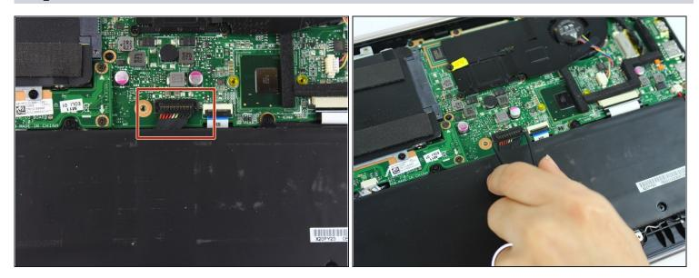
• Remove the ribbon cable with a pair of <u>tweezers</u>.
