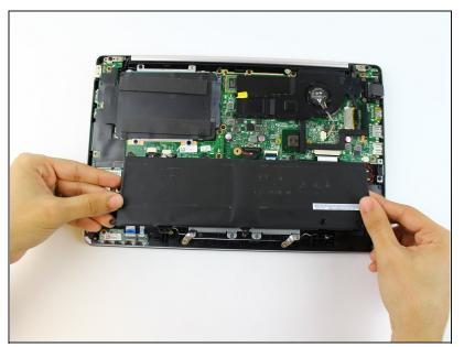
• Lift and remove the battery.
