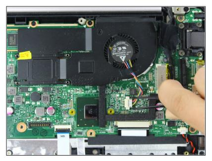
Disconnect the fan's power cable by pulling upward on the pin connector with a pair of tweezers.
