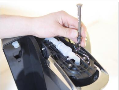
Remove the two 10mm Phillips #1 screws from the switch.
