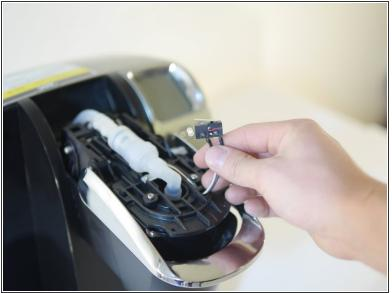
Remove the switch by cuting the two connecting wires. Reconnect a replacement switch <u>using this</u> <u>guide to join wires with solder</u>, or <u>using this guide to solder connections</u>, or by using any other technique to connect wires.
