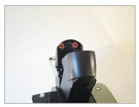
While looking upwards from underneath the Keurig, remove the two 8mm Phillips #2 screws from underneath the black plastic "shroud".
