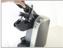
Remove the black plastic "shroud" by pushing inwards and then pulling upwards to disengage the plastic hooks that are not visible.
