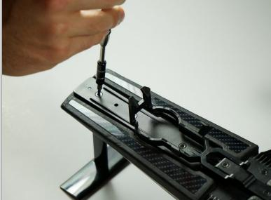
Remove the far left 1cm screw using a T8 screwdriver.
