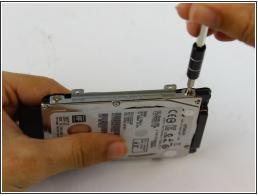
Remove two 3mm screws using a Phillips 0 screwdriver from each sides of the hard drive bracket.
