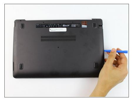
Use a plastic opening tool to pry the back panel off.
