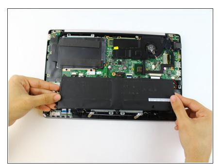
Lift and remove the battery.
