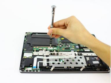
Remove four 4mm screws using a Phillips 0 screwdriver.
