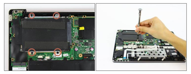
• Remove four 4mm screws using a Phillips 0 screwdriver.
