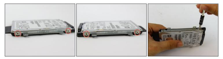
• Remove two 3mm screws using a Phillips 0 screwdriver from each sides of the hard drive bracket. The bracket should fall off after removal.
