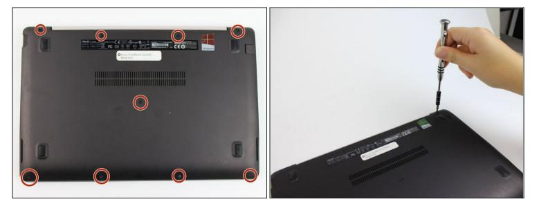
• Use a Phillips 0 screwdriver to remove nine Phillips screws from the back of the laptop (four 7mm from the top hinge, four 5mm from the bottom hinge, and one 10mm screw from the center).
