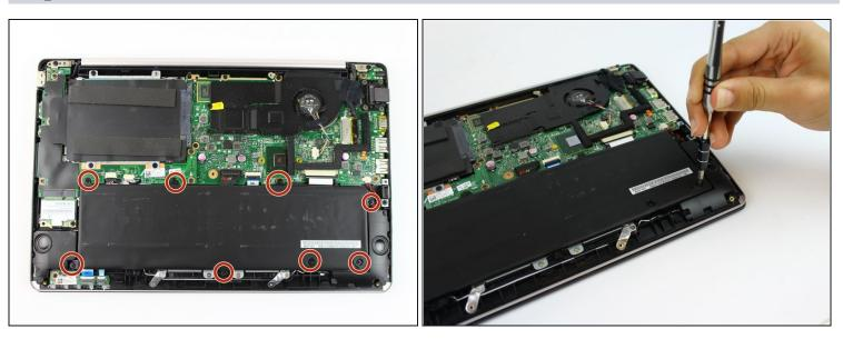
• Use a Phillips 0 screwdriver to remove the eight 5mm Phillips screws holding the battery in place.
