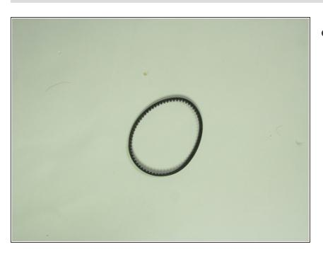
Replace belt if torn or damaged.
