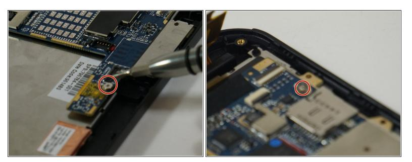
Remove the two 2 mm Phillips 000 screws from the motherboard.
