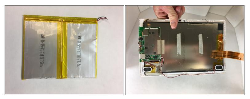
• The battery is now removed from the device. Replace the battery.
