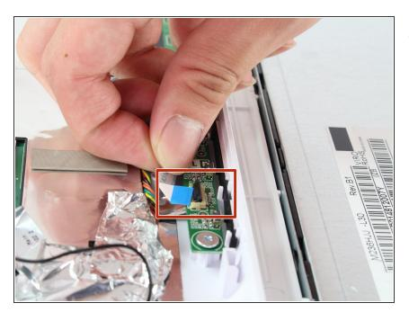
Remove the fiber cable with a blue tip by gently sliding it out.
