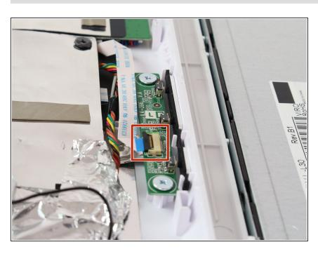
Lift up the black plastic tab holding the white fiber cable with the blue tip.
