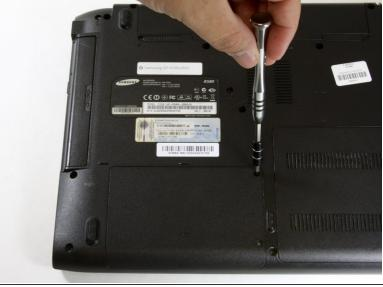
Remove both of the 5 mm Phillips head screws on the HDD back plate cover.
