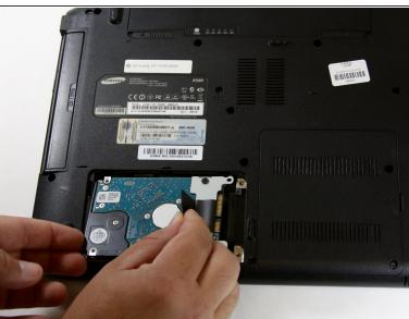
Grasp the tab and pull it to the left until the hard drive releases its connection and is able to be lifted free.
