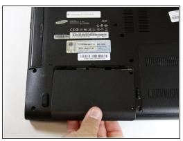
• Pull down while applying pressure to release HDD back plate cover and then lift the cover upward.
