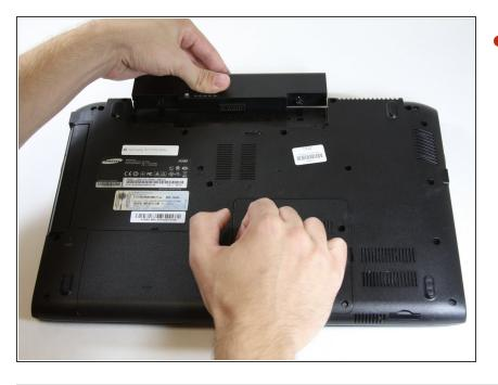
• Slide the battery pack upwards out of the battery housing.
