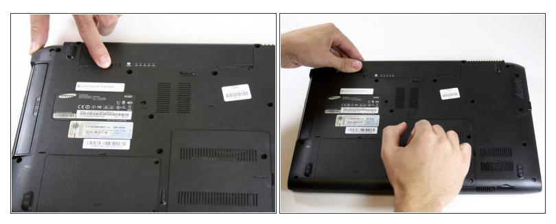
• Move the battery latches outwards into the unlocked position and grasp the battery latch.
