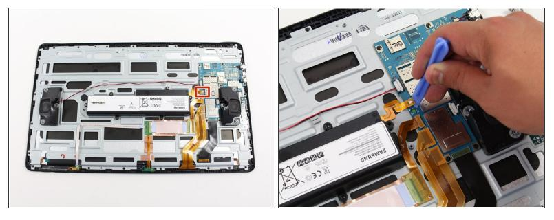
Using the plastic opening tool, lift off the orange press-fit connector (marked with a white arrowhead) where it attaches to the motherboard.
