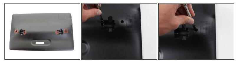
• Remove the 4 screws (4 mm in length) using the Phillips #0 screwdriver.
