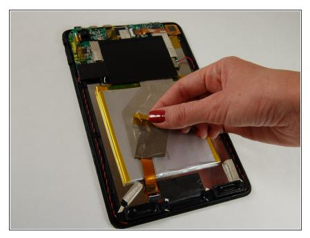
Start by placing tablet face down and carefully removing the mesh wire tap from the back of the battery.
