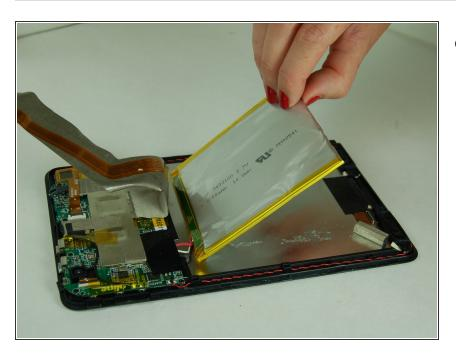
Remove battery and replace faulty one with new battery.
