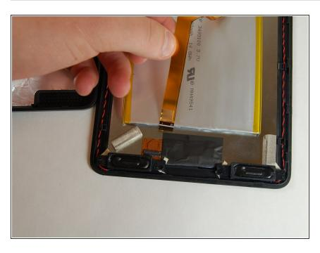
Remove the flat wire from its connector with the tweezers and fold to the side so that it's clear of the battery.
