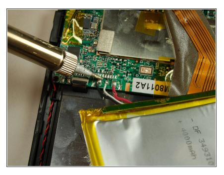
Once the soldering iron has heated up, begin by placing the tip of the iron where the wire directly meets the mother board. The soldering should heat up and allow you to gently pull the wire off. Repeat twice more to remove each of the three wires.
