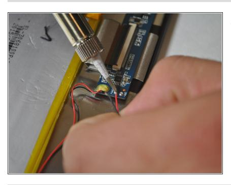
Remove wires from the device with a solder iron. Use the <u>soldering</u> <u>technique guide</u> for helpful tips!
