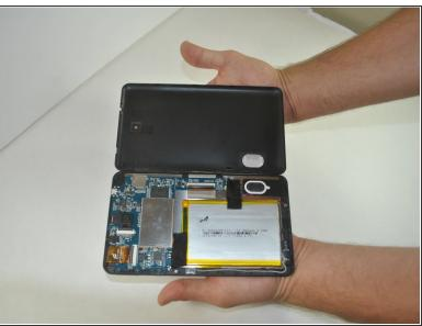
Separate the back of the device from the face by inserting the flat end of the nylon spudger into the corner of the device to safely pry it open.
