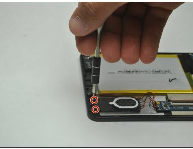
Remove the 4.1 mm screws connecting the speaker to the device by using the Phillips Head J #000.
