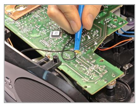
Scrape off the glue from the black wire with the blue plastic opening tool.
