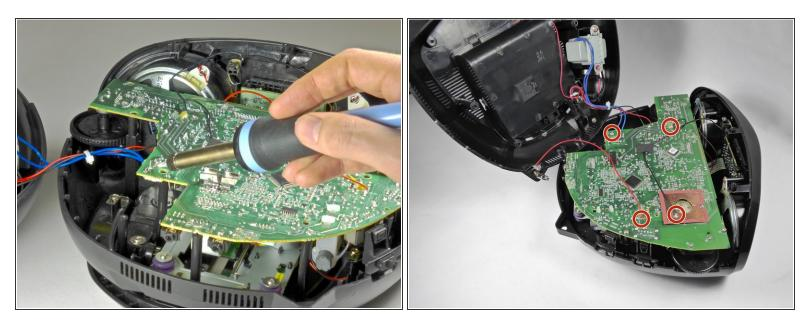
• Desolder the one black, one red, and two blue wires. If you need help soldering, see this guide.
