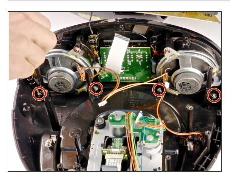
Remove the four 8.5mm chrome screws from the front panel with the Phillips PH1 screwdriver.
