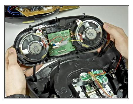
Remove the front panel from the top casing.
