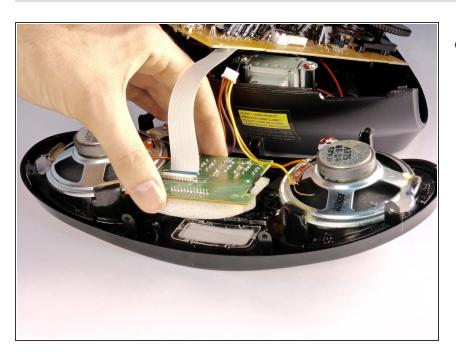
Lift the board to remove it from the front panel.
