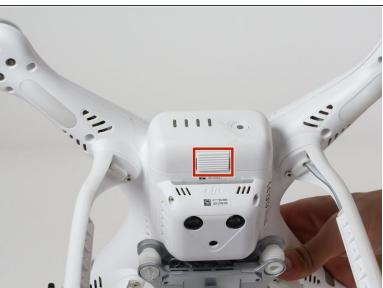
With the battery facing you, locate the two tabs on the top and bottom of the battery as shown.
