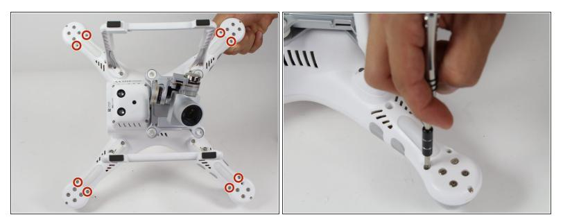
• Remove the eight 5mm long 2.5mm screws using the T-8 screwdriver.
