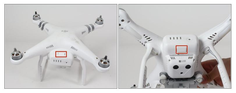
• With the battery facing you, locate the two tabs on the top and bottom of the battery as shown.
