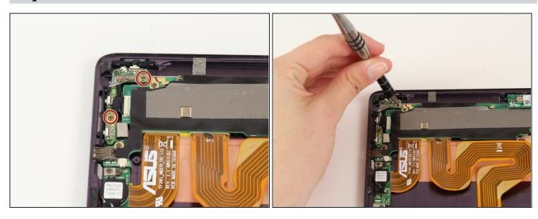
• Remove the two 2.5mm screws using a Phillips #00 screwdriver.
